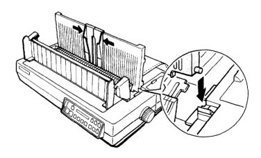
**9.** Pull the paper guide in the direction of the arrow in the illustration.
